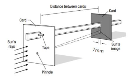
Move the cards on the meterstick until you create an image of the Sun that is exactly 7 mm wide. Fill in the data table below.
