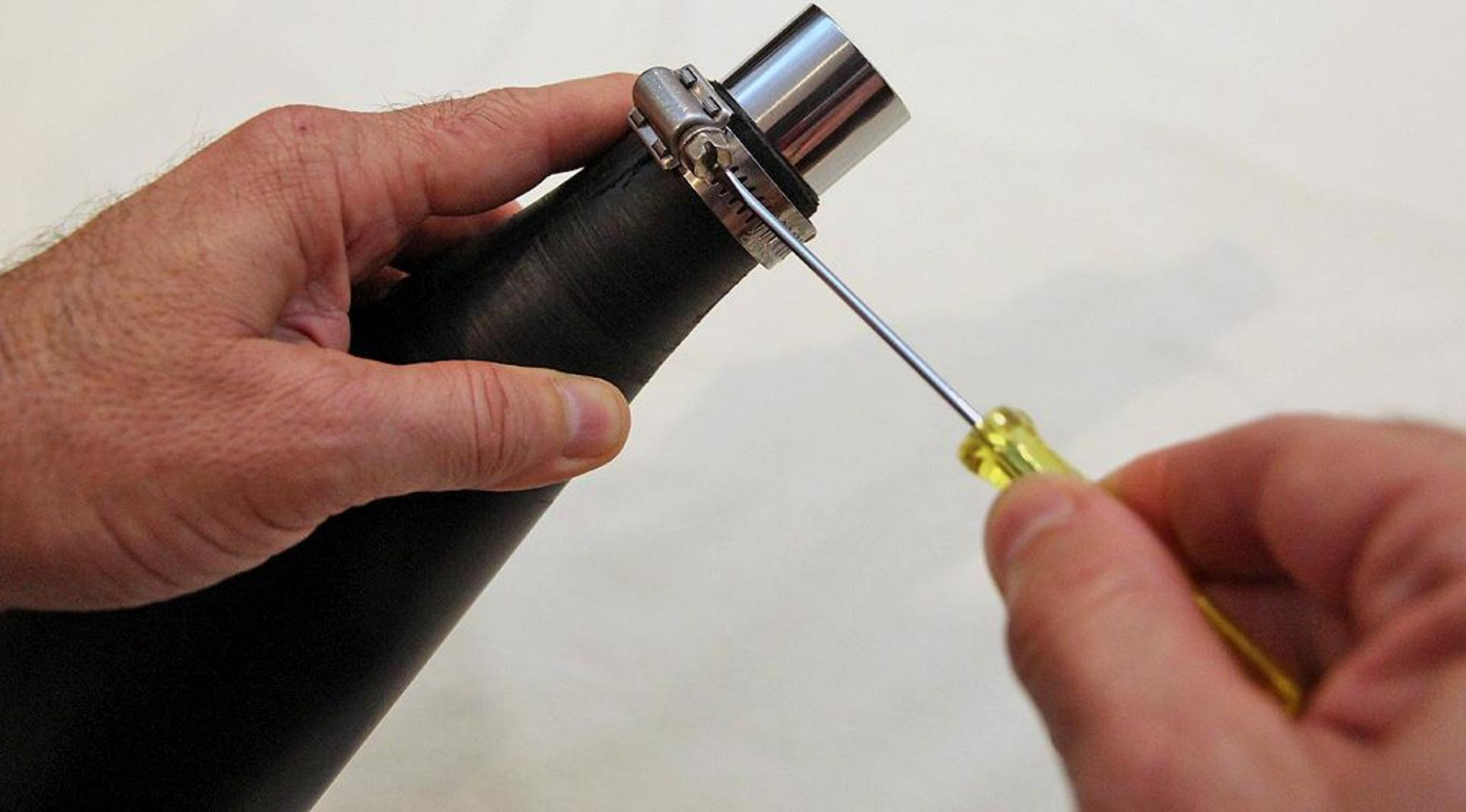
**Step 9.** Turn the funnel wide end up (you might find it easiest to sit in a chair and hold the funnel between your knees). Place the rear-projection screen (or two layers of vinyl shower-curtain liner) over the wide opening; it doesn't matter which side faces down. Lower the large hose clamp over the wide end of the funnel...
